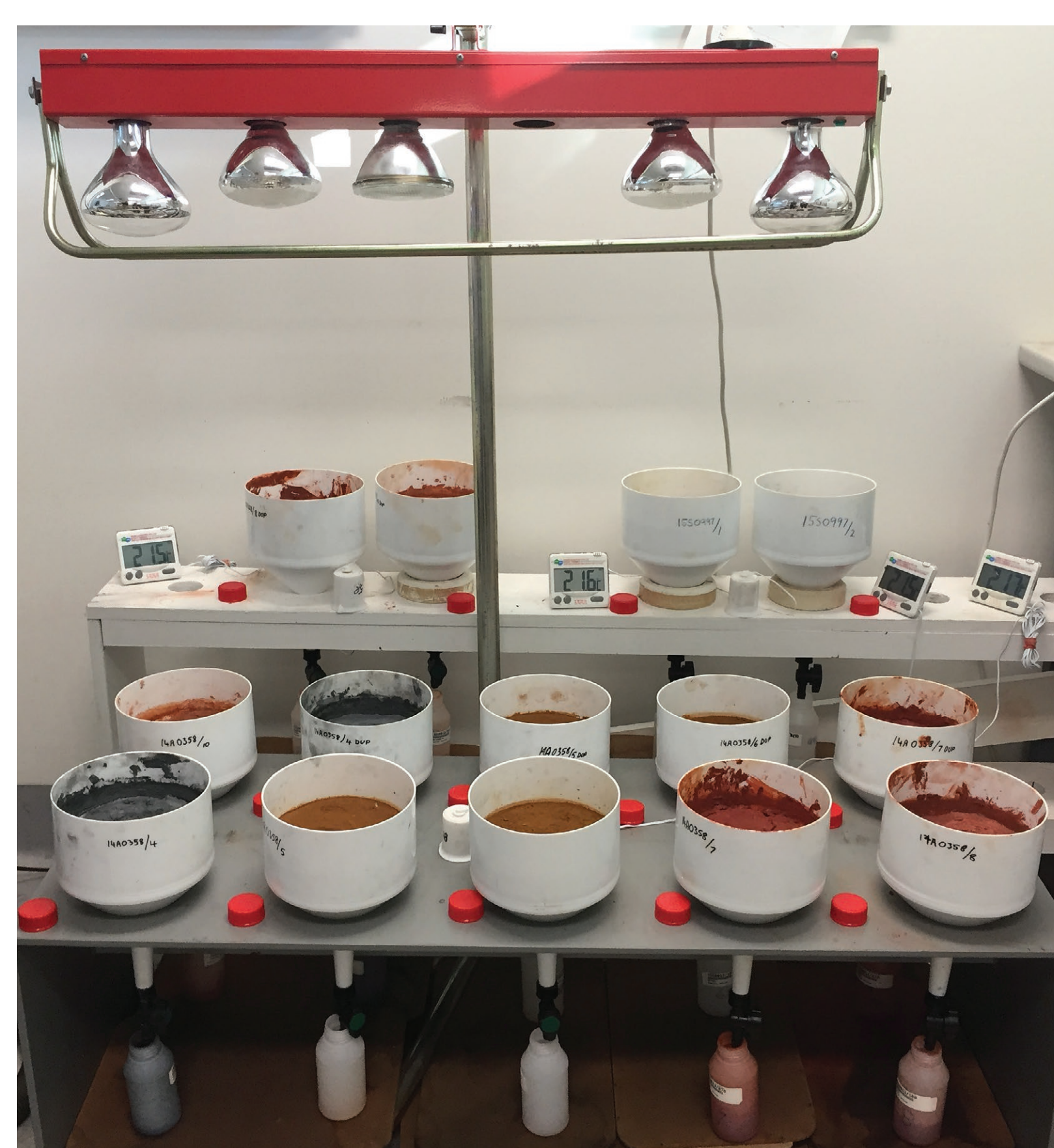
Fig.2. Kinetic Leaching Study over 24 months
